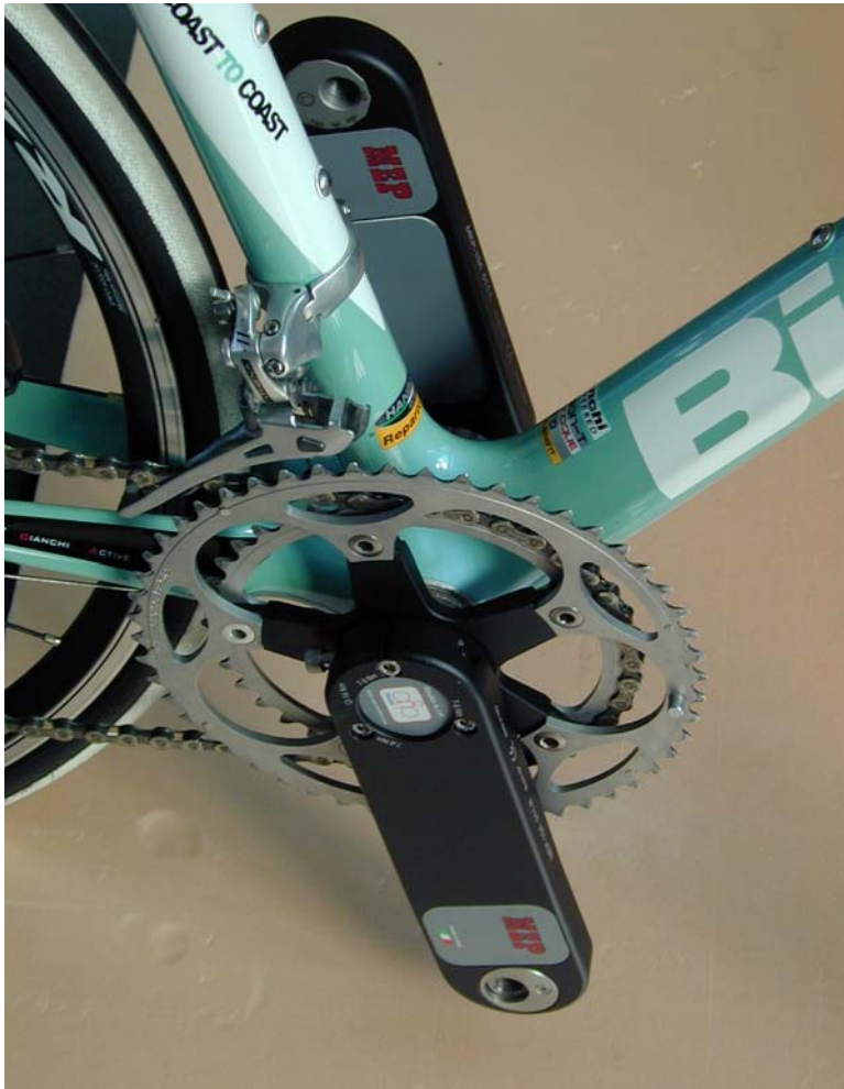
Figure 8 – Left crank arm inserted, MEP system fully assembled
