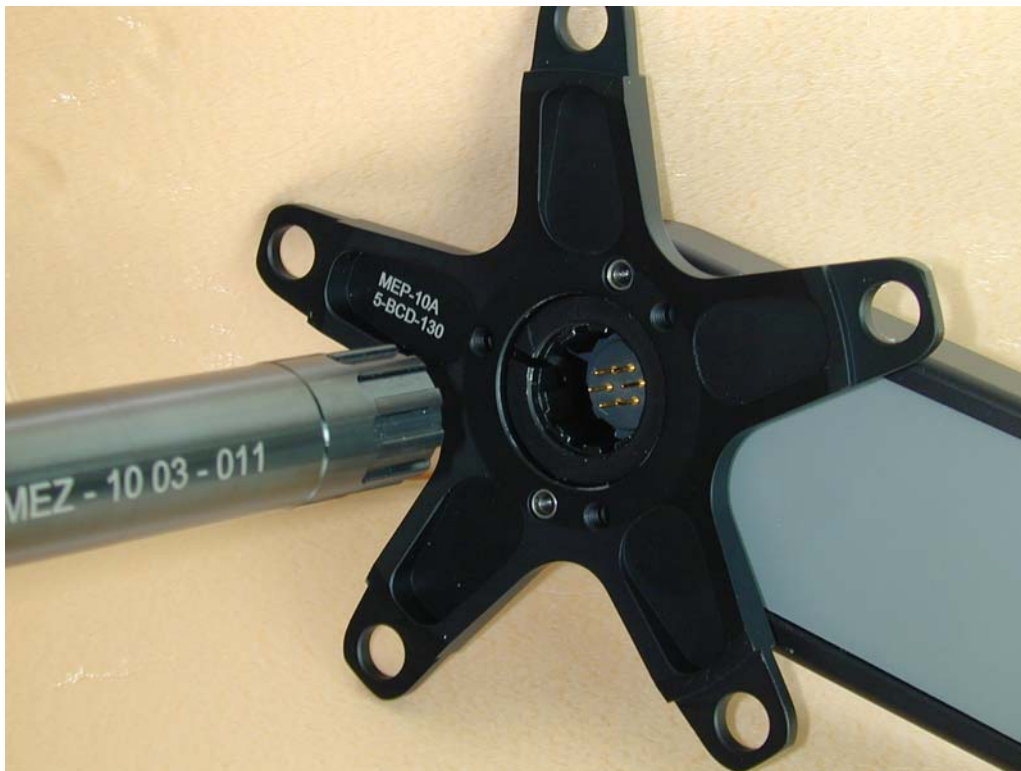
Figure 3 – Spindle set up on driving crank arm
