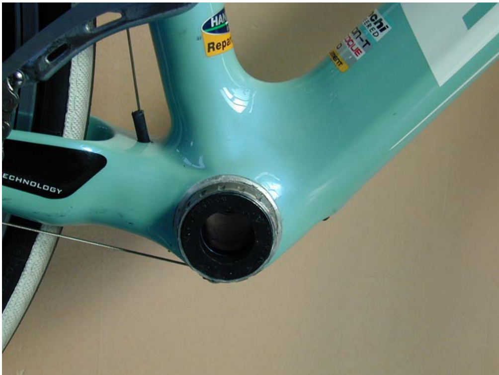
Figure 6 – Bike's look in BB shell zone just before MEP set up in place
