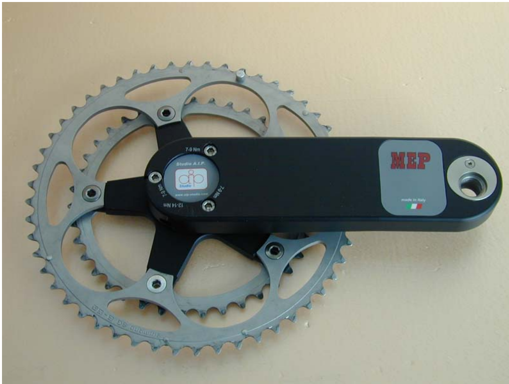
Figure 4 – Chainrings mounting on spider arms.
