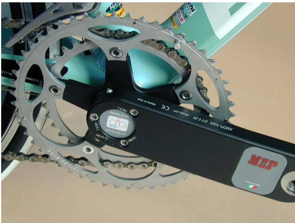
Figure 7 – MEP system into BB shell with external BB bearings
